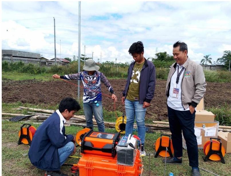
Photo 2. Laying out of wires and rods using the Schumberger Electrode array for georesistivity survey
