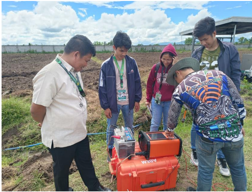
Photo 1. Preparation of the Vertical Electrical Sounding (VES) instrument at the survey site
